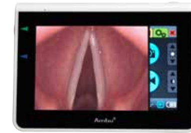
Image Extend enlarges the live image on aView™ for better viewing at a distance.
